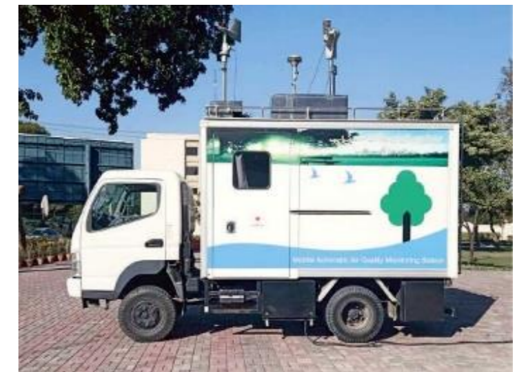
Figure 36: Mobile Air Quality Monitoring Truck (India)
